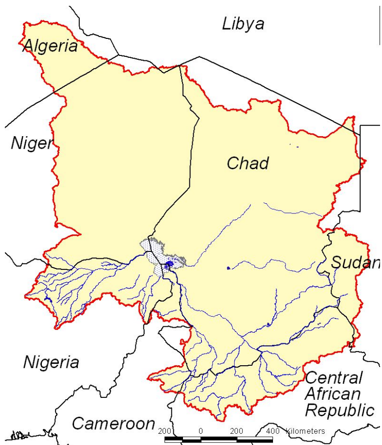
Figure 1.1 Lake Chad basin (yellow area) design based on HYDRO1K, a geographic database that provides coverage derived from the USGS' 30 arc-second digital elevation model of the world.
